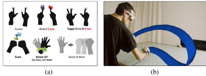
Figure 8.24: Gestures allow users to draw strokes using their fingers and arms. For example, (a) users draw with their fingers in AiRSculpt [33], and (b) with their arms in Surface drawing [101].
