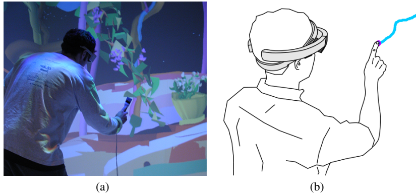
Figure 8.12: Follow-hand is the most common stroke creation interaction technique. (a) CavePainting [19], and (b) diagram of the interaction [16].
